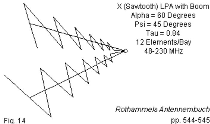
The specified design range for the array was 48 to 230 MHz. However, calculations of the element locations appear to have used a minimum design frequency of 50 MHz. The dimensions appear in **Fig. 15** in a 2-part table. The lower section shows the calculation of the boom positions for the array. The models for this array used 2.54-mm (0.1”) diameter lossless wire. **Table 5** samples the arrays performance at 50, 100, 150, and 200 MHz.
