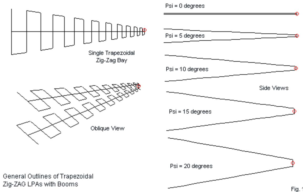
Early zig-zag LPAs generally used quite large values for  $\alpha$ , mostly for the practical reason of arriving at relatively short array boom lengths.  $60^\circ$  was perhaps the most common angle to appear in literature and commercial designs. Arrays also used  $\tau$ -values between 0.6 and 0.8 to reduce the element count and arrive at a lighter overall structure. (Most LPDA literature recommends no  $\tau$ -value below about 0.8, with higher values necessary to reduce the potential
