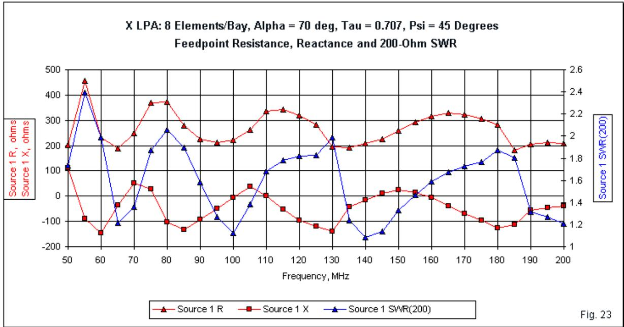
The impedance graph reveals that the small X LPA undergoes more radical changes in both resistance and reactance than the larger array. As well, we can easily find the SWR excursions above 2:1 at 55 and 80 MHz, with a borderline case at 130 MHz.
