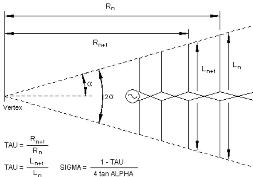
Log-Periodic Basics Applied to Dipole Arrays
