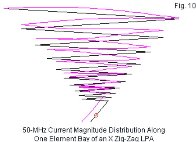
To allow more detailed comparisons between the trapezoidal and the X LPAs, we may look at sample data at 50, 100, 150, and 200 MHz for the range of  $\psi$ -angles covered by this initial exploration. The range of  $\psi$ -angles for the X LPA is not the same as for the trapezoidal counterpart. X arrays have been successfully used when  $\psi = 0^\circ$ , with a small separation between the bays. In fact, we shall later discover that a  $\psi$  of  $10^\circ$  may be the most optimal angle
