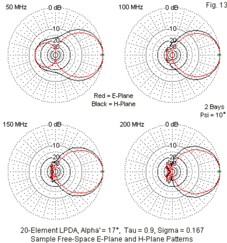
To go with the data on the E-plane and H-plane beamwidths, **Fig. 13** presents combined free-space patterns for the version using a  $\psi$ -angle of  $10^\circ$ . As we increase the value of  $\psi$ , the H-plane beamwidth decreases with almost no effect upon the E-plane beamwidth. At an angle of  $15^\circ$ , the two beamwidth values are virtually equal.
