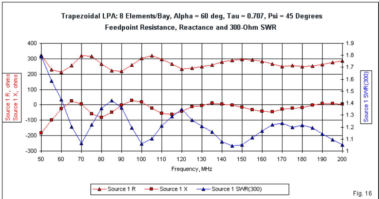
One of the factors limiting array performance is the use of a very high value for  $\psi$  ( $45^\circ$ ). Early trapezoidal LPAs tended to use  $\psi$ -angles between  $35^\circ$  and  $45^\circ$  in order to assure the highest gain from the fewest elements. The present example is no exception. Without further
