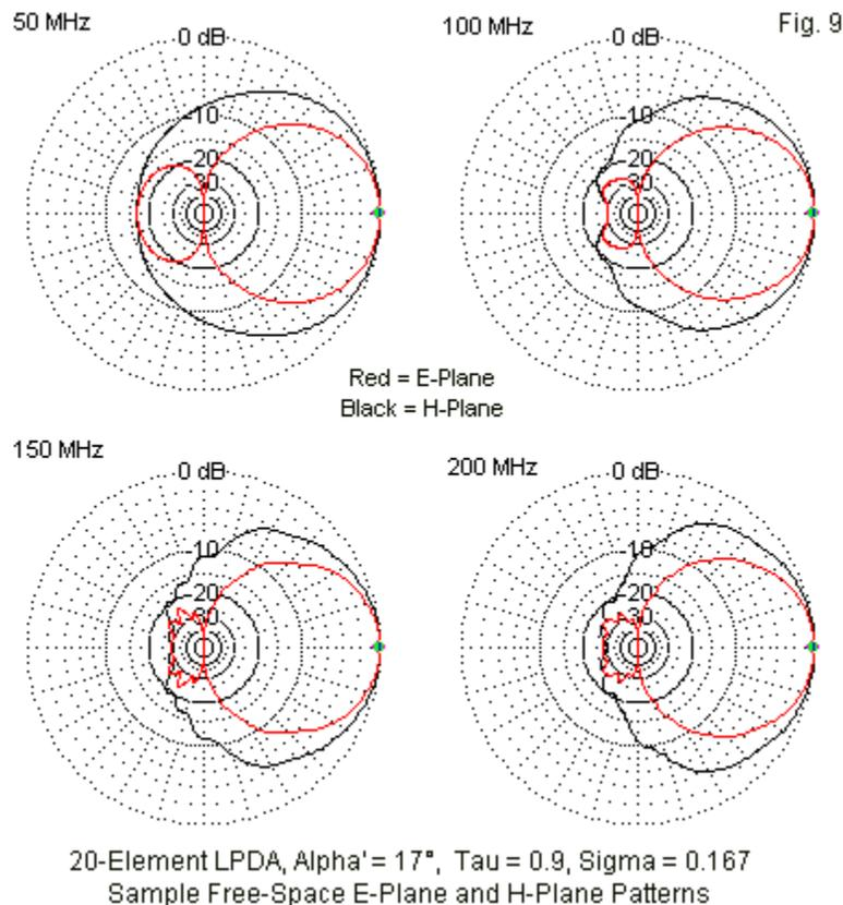
In **Table 2** are the summary values derived from a frequency sweep across the entire operating passband in 5-MHz increments.
