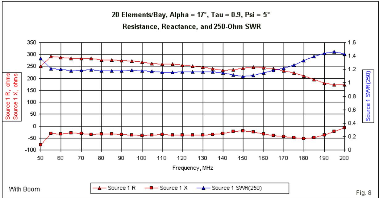
Very little distinguishes the performance of boom-equipped trapezoidal LPAs and their X counterparts, once we compensate for any deficiencies at one or the other end of the operating passband. One might profitably study the corresponding data for all  $\psi$ -angles for both types of arrays in the data appendix.
