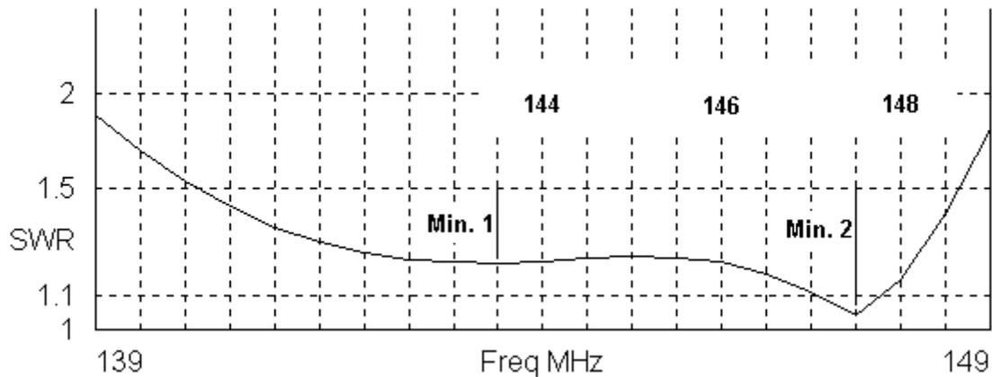
**Fig. 3** presents the 50-Ohm SWR curve for the array from 139 to 149 MHz. The curve is typical of optimized OWA designs. (Yes, even an optimized wideband antenna may be optimized within its overall design parameters.) Most noticeable and telling is the presence of two dips in the SWR, one shallow dip at 143 MHz and one very sharp dip near 147.5 MHz. The rise in SWR above 148 MHz is very steep, while below the operating passband for the antenna, the SWR rises very slowly.
