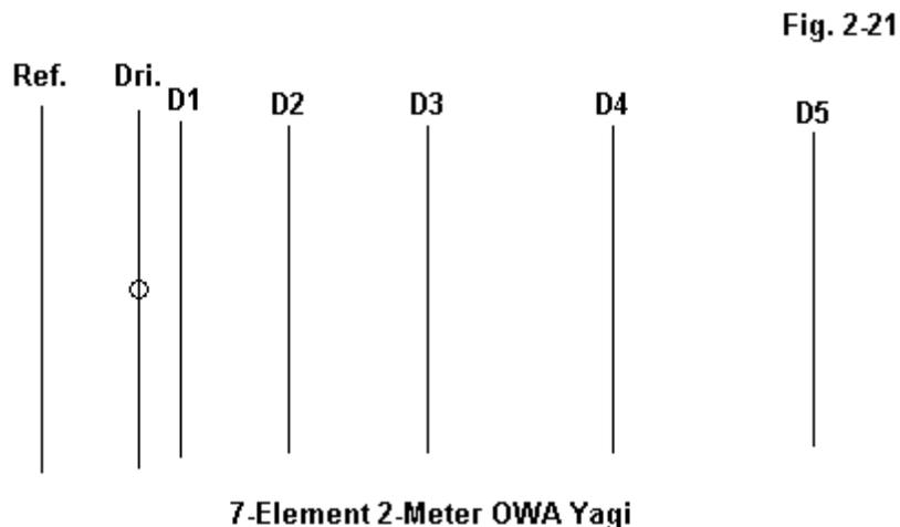
**Table 8** provides the dimensions of a 7-element 2-meter OWA Yagi that is quite capable of forming the basic unit for a family of 2-meter OWA Yagis. The outline appears in **Fig. 21**. The design improves upon the 6-element OWA--itself a perfectly good antenna--by optimizing the element spacing for the 0.1875" elements. Since these elements are larger in diameter--
