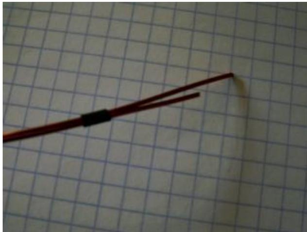
**Figure 9b.** A trick to identify the specific wire by making it a bit longer at both ends
