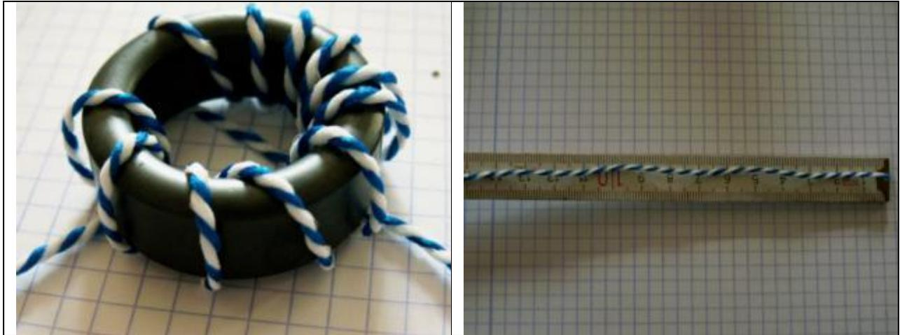
**Figure 9a.** How to determine the wire length
